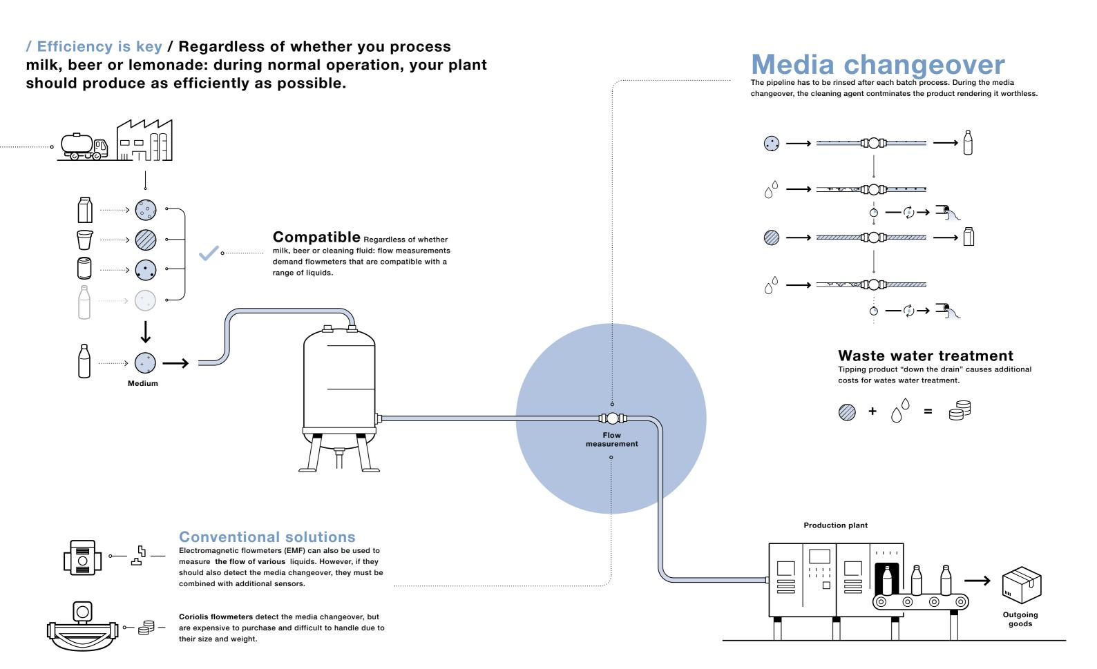
/ Flow measurement with SAW technology / Hygiene is the top priority when producing food products and beverages. FLOWave provides you with a compact solution that meets strict hygienic requirements. Thanks to innovative SAW technology, the flowmeter dispenses with sensor elements in the measuring tube. No parts in the measuring tube means: no leaks, no material incompatibility, no maintenance, no pressure drop and easy cleaning.
